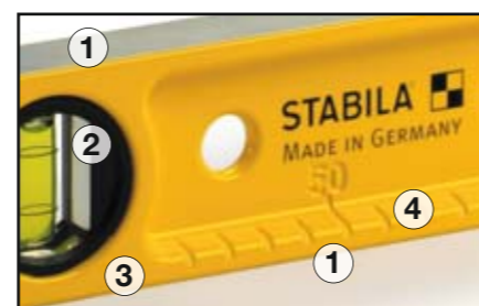
1 Two milled measuring surfaces for easy use in every situation. 2 Securely cast-in vials. The STABILA patent makes recalibration superfluous. 3 Measuring accuracy in the normal position ± 0.029° = 0.5 mm/m. 4 Abrasion-proof scale with measurements displayed in cm. 5 Large hand holes – easy handling.
