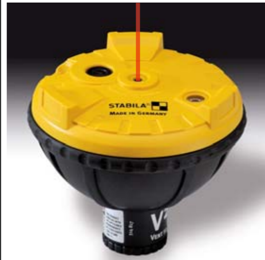
V2R: Its hemispherical shape allows it to be easily aligned in the pipe using the illuminated circular vial; the laser transmits its plumb-line up to the roof at the touch of a button.
