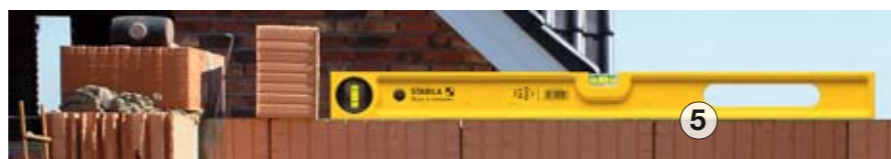
1 Two milled measuring surfaces for easy use in every situation. 2 Securely cast-in vials. The STABILA patent makes recalibration superfluous. 3 Measuring accuracy in the normal position ± 0.029° = 0.5 mm/m. 4 Abrasion-proof scale with measurements displayed in cm. 5 Large hand holes – easy handling.
